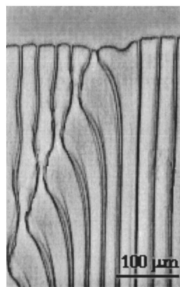
FIG. 28. Solitary tilt wave in a hypoeutectic sample. Same run as in Fig. 10(b).
